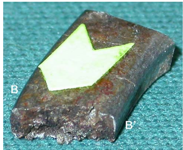
Fig. 7 Photograph of fresh fracture surface generated by breaking open along pre-existing cracks in hanger (Fracture B–B', shown in Fig. 2)
