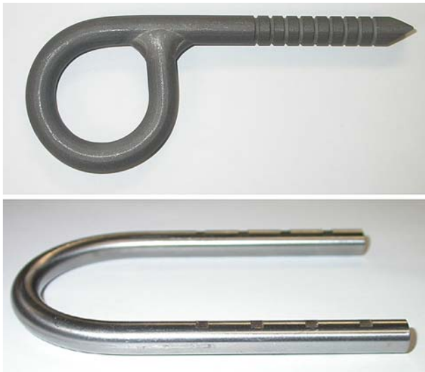
Fig. 10 Photographs of glue-in titanium bolts used for fixed climbing protection; unalloyed welded titanium (top) and Ti–6Al–4V U-bolt (bottom)
