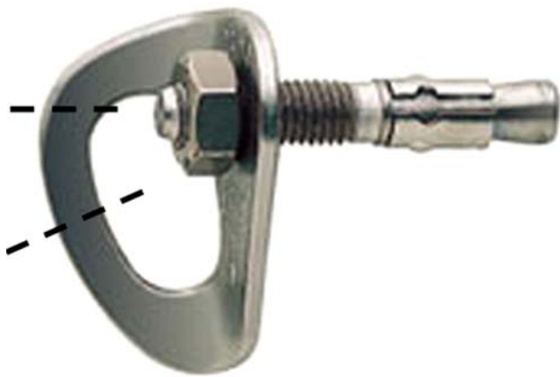
Fig. 1 Photograph of typical rock climbing bolt used for fixed protection an austenitic stainless steel expansion bolt, nut, and 316L hanger (most common). Dashed lines indicate fragment recovered after failure and available for analysis
